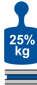
Horizontally mounted = 25% quoted load rating
